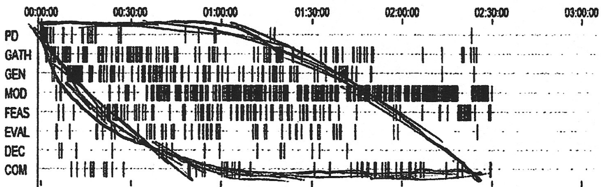
Figure 1: Example of expert cascade pattern (Borgford-Parnell, Deibel, & Atman, 2010). Note the progression from the upper left to the bottom right. The cascade pattern, or “Ideal Project Envelope,” begins in Problem Scoping, transitioning between Problem Definition (PD) and Information Gathering (GATH); then progresses to Developing Alternative Solutions, transitioning between Generation of Ideas (GEN), Modeling (MOD), Feasibility of Analysis (FEAS), and Evaluation (EVAL); and throughout the process transitions to Problem Scoping and Project Realization, which includes Decision (DEC) and Communication (COM).
